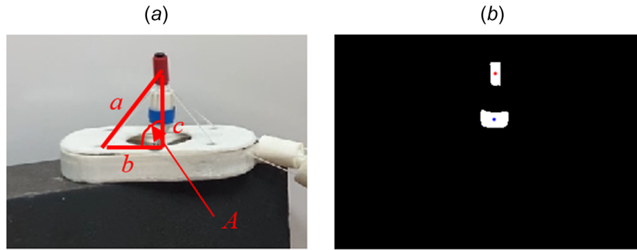
Fig. 9 MATLAB video analysis of tool movement about the y-axis
